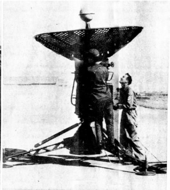
McQueen, a member of an Air Force mobile weather team. As the balloon sails into the sky, Airman McQueen and Team Chief Master Sergeant Dow Sherry, direct an automatic tracking antenna (center) onto the trail of the balloon to
