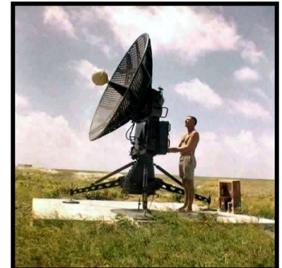
Big Jim Fraser testing tracking on GMD-1 at Malden
